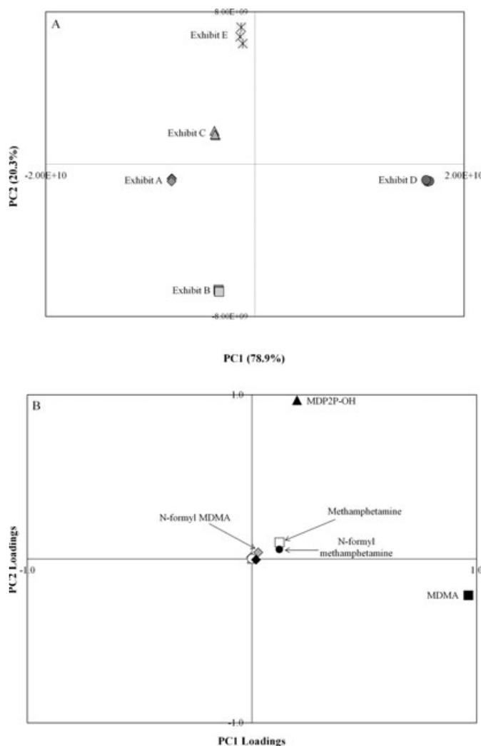
FIG. 7—Principal components analysis (A) scores plot and (B) loadings plot for five methylenedioxymethamphetamine exhibits extracted using head-space solid-phase microextraction and analyzed using Temperature Program 2. Each exhibit is labeled in the scores plot and selected compounds are labeled in the loadings plot.
