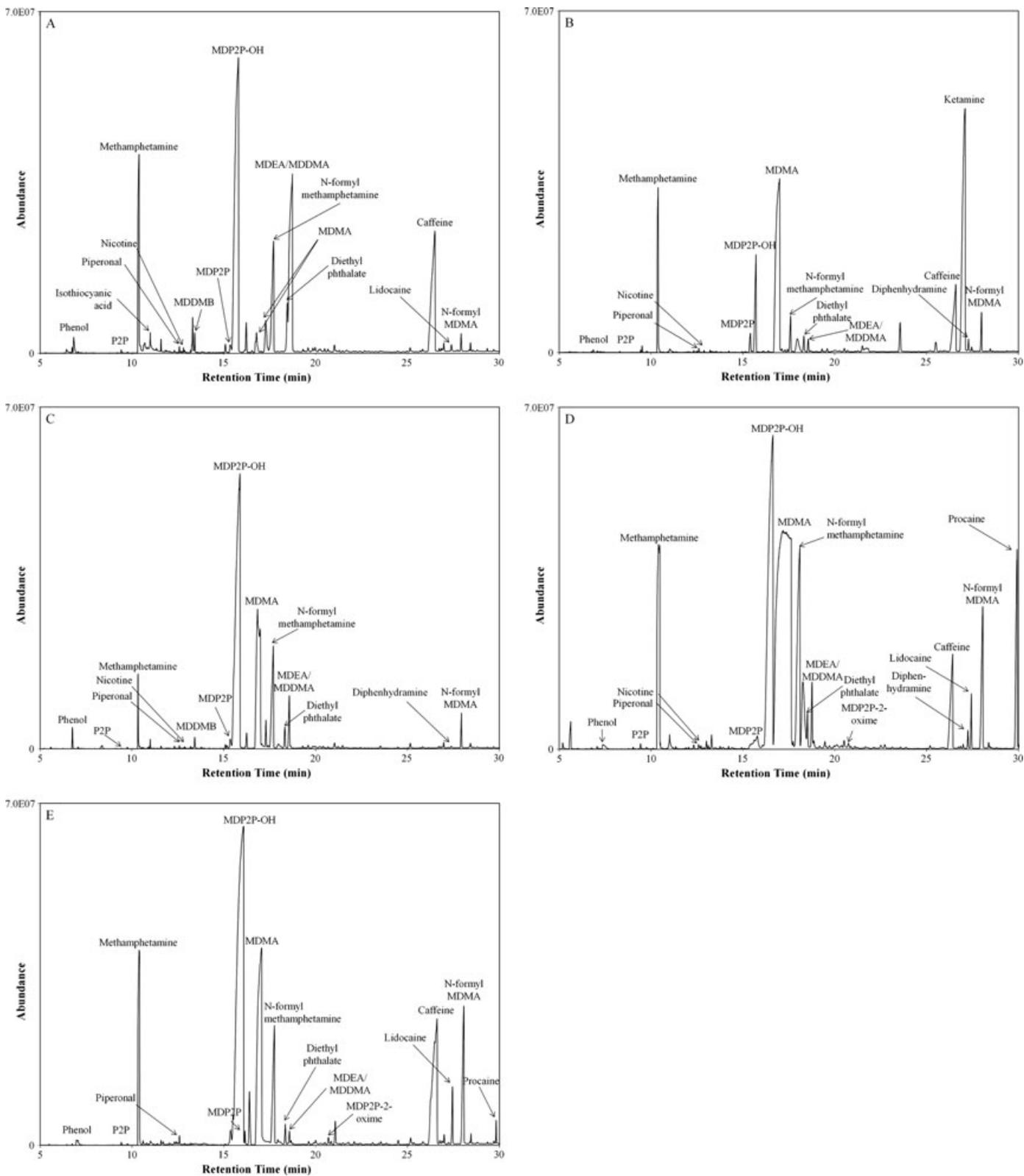
FIG. 5—Total ion chromatograms for five methylenedioxymethamphetamine exhibits extracted using headspace solid-phase microextraction and analyzed using Temperature Program 1 (A) Exhibit A, (B) Exhibit B, (C) Exhibit C, (D) Exhibit D, and (E) Exhibit E. Peaks are labeled with provisional identities based on a mass spectral database search.
