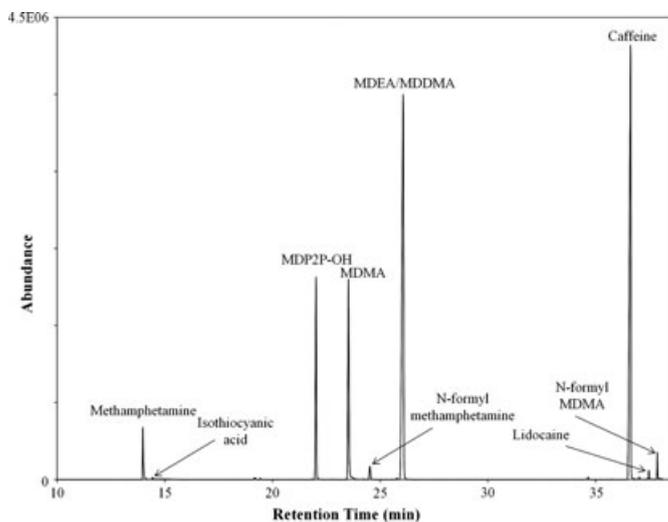
FIG. 2—Total ion chromatogram of Exhibit A extracted using liquid-liquid extraction and analyzed using Temperature Program 2.
